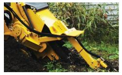
MAKE SENSE OF YOUR TRENCH. When difficult ground conditions are encountered, causing a sudden drop in engine speed, AutoCreep automatically pauses and the tractor slightly backs off the forward trench wall to prevent an engine stop. Once the preset engine and trencher speed recover, forward AutoCreep resumes. The TrenchSense<sup>™</sup> electronic control sequence occurs within seconds and requires no operator adjustment to the controls.
