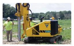
**COMPACT DESIGN.** A small machine with operating dimensions of 12.5' (3.8 m) wide, 19.6' (6 m) tall and a 15' (4.6 m) mast is ideal for jobsites with less space, or for multiple smaller jobs that require continual transportation of the machine. Quickly move around the jobsite and continue efficiency of installations, helping reduce time spent on setup, teardown and transportation.
