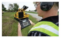
**TAKE CONTROL.** With a wireless remote, crews can operate the PD5R and gain visibility around the machine, while controlling most machine functions like hammer engagement, pile accuracy, auto plumb and ground drive, all while remaining out of an operator's seat during installation.
