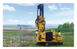
**KEEP IT LIGHT.** The PD5R weighs in at 10,300 lb (4672 kg), which allows for transporting up to two pile drivers on select trailers, and less potential damage to jobsites, all while helping increase efficiency of setup and teardown with a lightweight design.
