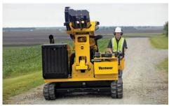
**KEEP IT LIGHT.** The PD5 weighs in at 10,350 lb (4694.7 kg), which allows for transporting up to two pile drivers on select trailers, and less potential damage to jobsites, all while helping increase efficiency of setup and teardown with a lightweight design.
