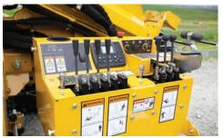
ON-MACHINE CONTROL. Walk-beside, machine-integrated controls allow the operator to control machine functions, including engagement of hammer, pile placement and ground drive. Operators remain off the machine and walk beside
