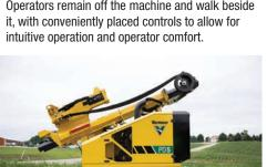
**COMPACT DESIGN.** A small machine with a width of 12.5' (3.8 m), a height of 19.6' (6 m) and a 15' (4.6 m) mast is ideal for jobsites with less space, or for multiple smaller jobs that require continual transportation of the machine. Quickly move around the jobsite and continue efficiency of installations helping reduce time spent on setup, teardown and transportation.
