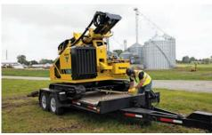
TRANSPORTATION EASE. Teardown and transporting is convenient with a rotating platform and a mast that can stay fully assembled and stow parallel with the tracks, making it more convenient for the entire crew to move to the next job.
