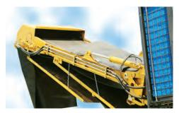
**LOADOUT CONVEYOR.** A smooth discharge conveyor belt, equipped with a scraper that cleans the belt as it passes back to the mill box, reduces material buildup on the belt. Dual chutes help to separate shingle dust from nails.
