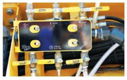
WATER APPLICATION SYSTEM. Adding water during the grinding process helps to extend the life of the cutters and other wear surfaces, and reduces the amount of dust and shingle residue on the machine components.
