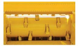
**DUPLEX DRUM.** The patented Series II duplex drum system improves cutting performance, and reversible hammers and tips simplify maintenance and nearly double wear life.
