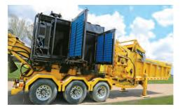
**COOLING AND FILTRATION SYSTEM.** The cooling and filtration system is specially designed to reduce the amount of dust that is pulled into the cooling package. Wide fin spacing and filters are designed to reduce the buildup of dust and tar on the cooler surfaces, and swing-out doors allow for easy ground level access for cleaning and filter replacement.
