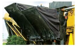
**AIR INTAKE.** The cooling package air intake chutes are located high on the machine to provide more clean air and less dirt-contaminated air from near the ground.
