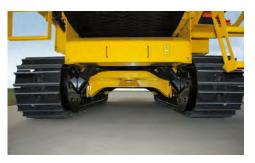
**MOBILITY.** The track-driven grinder offers onsite mobility with a remote control. The HG4000 $\pi$ x is designed with 16" (40.6 cm) of ground clearance, enhancing the unit's ability to traverse difficult terrain.
