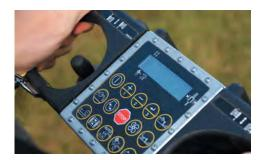
**REMOTE CONTROL.** A state-of-the-art wireless remote control unit allows the operator to run most machine functions from up to 300' (91.4 m) away.
