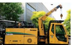
OPERATOR-CONTROLLED ROD LOADER. Helps reduce the labor involved with manually loading and unloading drill rod which also assists in increasing overall drilling efficiency.
