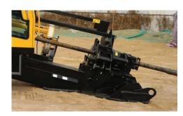
**OPTIONAL FRONT-MOUNTED STAKEDOWN** SYSTEM. Helps reduce the amount of time and materials needed to set up and secure the drill for enhanced jobsite efficiency.
