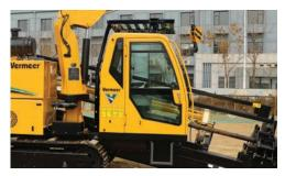
**CLIMATE-CONTROLLED CAB.** Enhances operator comfort and provides protection from the weather, which reduces operator fatigue and discomfort, helping you be more productive.
