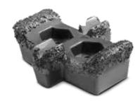
**WING TIPS.** Wing tips have a unique design with an overlay of carbide that provides an effective solution for processing large-diameter woody material — a narrow center section helps the tip penetrate the log, then the wings clean out the remainder. Wing tips can be flipped for double the life. **PN 296367135** shown
