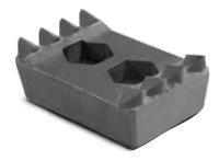
**IMPACT-RESISTANT TIPS (I/R).** Impactresistant tips offer an alternative to wing tips and are used to process large-diameter material. Their carbide inserts are very hard but also brittle, and are not intended to be used when contaminants are prevalent. I/R tips are cost-effective, offering dual side use. **PN 180012617** shown
