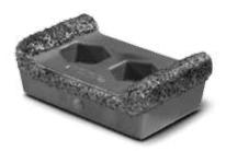
wide block tips. Wide block tips are the most common in the industry. They can be used in a variety of applications such as land clearing, regrind, pallets, compost and green waste. Wide block tips can be flipped for double the life.
