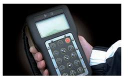
**OPTIONAL REMOTE CONTROL.** Operate one machine to load while still maintaining control of the chipper. The remote control operates forward, reverse and stop functions of the feed rollers, restarting the feed rollers, engine throttle, engine stop, crush boost for the upper feed roller and hydraulic discharge chute positions (if equipped).
