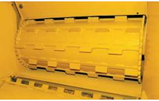
**LOWER FEED ROLLER.** The lower feed roller is offset from the upper feed roller by 11" (27.9 cm). Material is easily pulled to the upper feed roller, so there is less need to manually raise the upper feed roller for larger diameter material.
