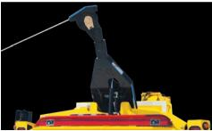
**OPTIONAL PATENT-PENDING WINCH.** Eliminates the need to drag large material to the chipper. The 150' (45.7 m) winch line can handle material up to 4000 lb (1814.9 kg), making it easy to lift logs directly onto the feed table. In addition the winch can also be hydraulically raised out of the way to allow operators to feed the unit using a loader.
